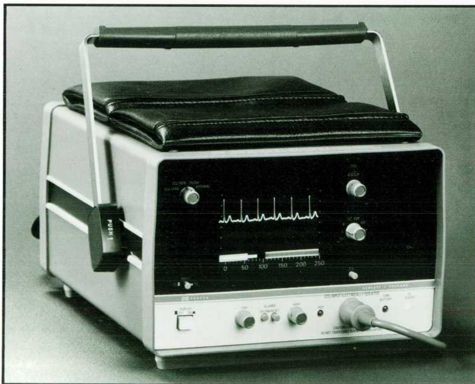
Fig. 1. Model 78333A ECG Monitor displays ECG waveform and heart rate with minimum interference from electrosurgery equipment or other sources of electromagnetic radiation. Internal rechargeable batteries can power the instrument for up to six hours.
